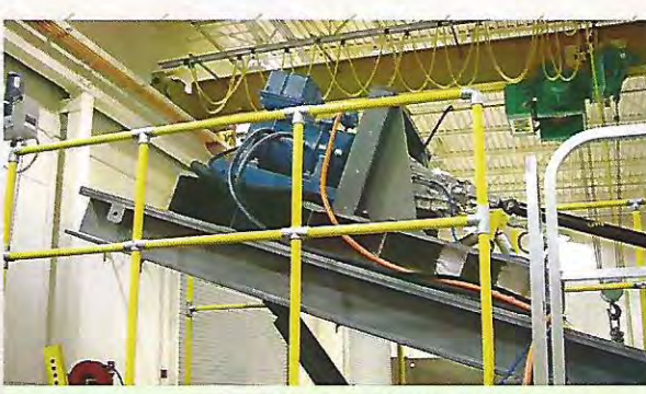
Southwest Research USA (Tilt & Roll Test Stand)
